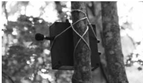
Figure 1. The SM2-Bat recorder.
